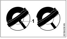
Left: Bottom of cap is twisted – inner mark (1) in line with outer mark.
