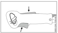
► Press down the throttle trigger lockout and open the throttle – the choke knob moves to the run position — After a cold start, warm up the engine by opening the throttle several times.
