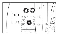
This setting provides an optimum fuel-air mixture under most operating conditions.
