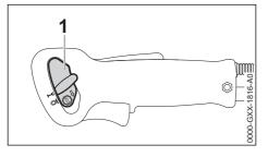
The slide control (1) is in the normal run position  ${\bf I}$ .
