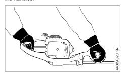
Left hand on the control handle, right hand on the cutterbar handle. Wrap your fingers and thumbs around the handles.
