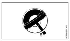
The marks on the tank cap and fuel tank are then in alignment.
