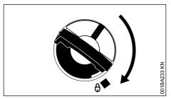
While holding the cap depressed, turn it clockwise until it engages in position.
