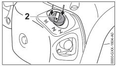
► Depress the outer ring (arrows) of the choke knob (2) and then turn it to <u>✓</u>.
