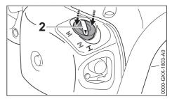
► Depress the outer ring (arrows) of the choke knob (2) and then turn it to <u>f</u>.
