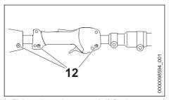
► Tighten down the screws (12) firmly
