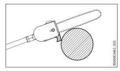
When performing the separating cut, position the bar against the branch near the hook. This will prevent the power tool from making jolting movements when you start the separating cut.
