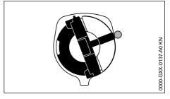
Markings on fuel cap and oil tank must align
