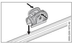
Squeeze the ends (arrows) together and push carrying ring onto the shaft.
