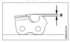
The depth gauge determines the height at which the cutter enters the wood and thus the thickness of the chip removed.
