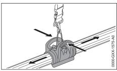
Squeeze the clip (carrying ring) together to move it up or down the shaft
