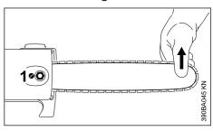
Re-tensioning during cutting work:
