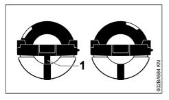
Left: Base of fuel cap is tilted – interior marking (1) is aligned with the exterior marking
