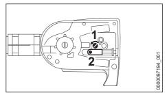
Turn the screw (1) counterclockwise until the tensioner slide (2) butts against the left end of the housing slot, then back it off 5 full turns
