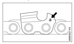
The chain pitch (a) is marked on the depth gauge end of each cutter.
