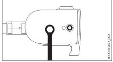
Unscrew the nut and remove the cover
