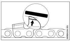
File the top of the depth gauge parallel to the stamped service marking (see arrow) – but do not lower the highest point of the depth gauge in this process.
