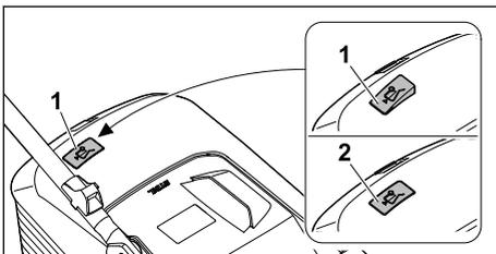
The flow of air generated by the blade raises level indicator (1). The flow of air stops when the grass catcher box is full. If the flow of air is too low, level indicator (2) returns to its resting state. This is a prompt to empty the grass catcher box.
